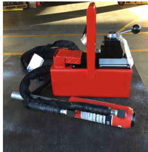
CABLE TENSIONING CT10
